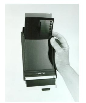
attenuation at all, and by placing a piece of light-proof black tape over a small area to completely block light from reaching the film. This area on the negative will then be my "film base plus fog" reference.
