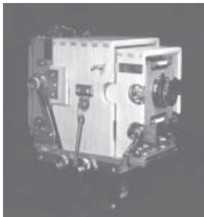
Figure 1. My Zone VI 4x5 camera is shown here with the wind enclosure attached. The rear section of the enclosure is attached to the back by brass brackets that fit under the knurled knobs that control back tilt, and is held firmly to the camera base by a small bungee cord. The front of the enclosure telescopes inside the rear section is tapered to allow bellows clearance, and attaches to the lens board by brackets that fit under the lens rise/fall/tilt knobs. Two thumbscrews secure the back and front sections to each other after focusing, creating one rigid film/lens configuration. Although most camera movements are eliminated by this design, sufficient movements are still allowed for the task at hand: making photographs of rime in the wind.
